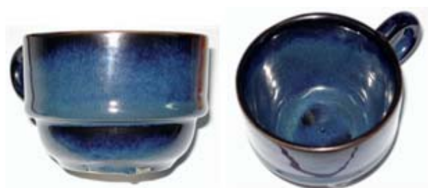
Textures of the waste containing glazes at various EAF dust to frit ratios (left) and over a ceramic body (right)
