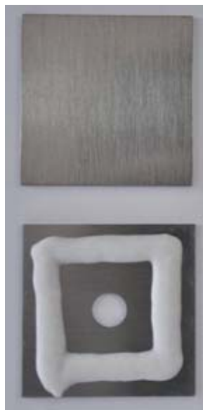
Glass paste on Crofer 22 APU plate for preparing sandwich specimen
